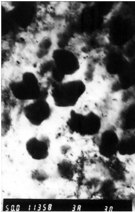
Fig. 6 The coarsened precipitates inside the recrystallization grains
