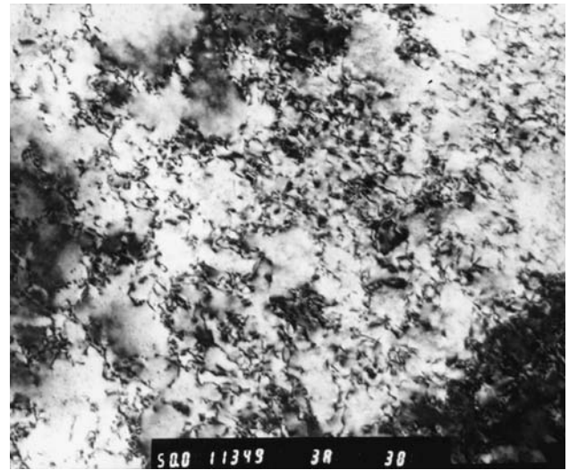
Fig. 5 Dislocations in 45% deformed specimen after aging at 500 °C for 1 h
